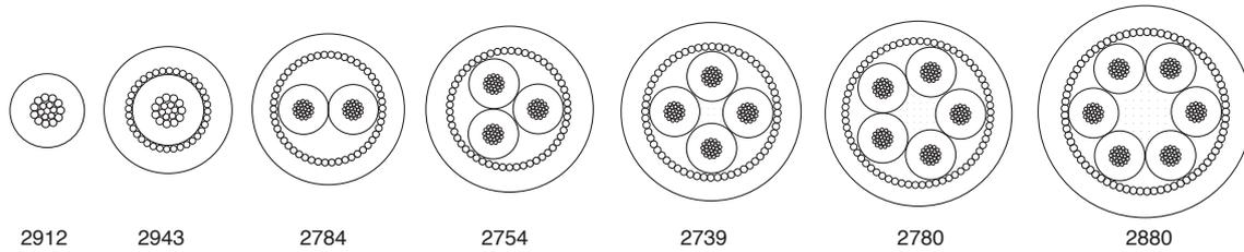
Most of these miniature cables were originally developed one by one as custom cable for a magnetic head lead which must be swiftly moved to specified position precisely by small energy such as a floppy disk drive. And then, some of them remained as continued items close to standard stock products, finding out unfixed varied demand in long period of time. For such application, these cables are indispensable, even thanked.
