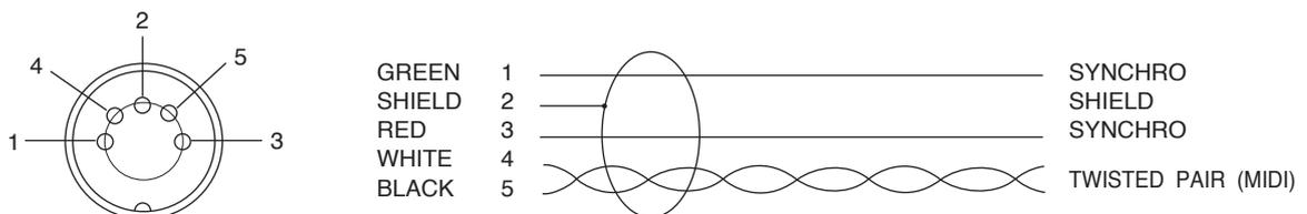
NOTE : Transmission lag in MIDI systems is mainly caused by the speed of the photocoupler and the rise time of the driver rather than the transmission characteristics of the cable.
