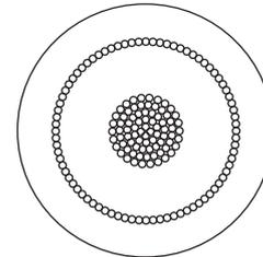
This standard speaker cable is designed to meet XLR audio connector cable clamp. Coaxial Design is used to provide as large a conductor size as possible, which results in the following features.
