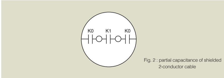
Fig. 2 : partial capacitance of shielded 2-conductor cable
