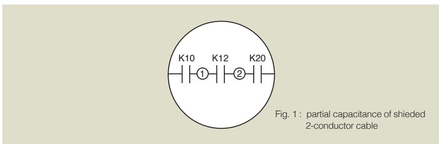
Fig. 1 : partial capacitance of shielded 2-conductor cable
