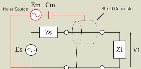
Fig. 4: Electrostatic Shield
