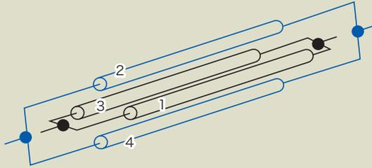
Fig. 7: Cancellation of electromagnetic coupling by star-quad connection
